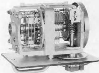
Figure 8. Interior view of the Type 1422-ME, a dual-range unit, calibrated in capacitance removed, 0 to 10.5 and 0 to 105 pf.
