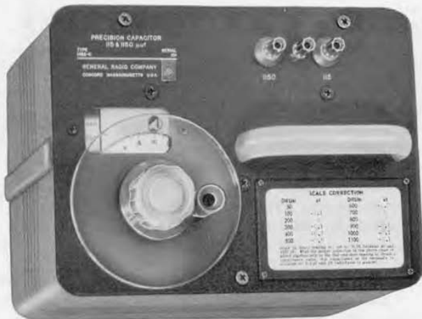
Figure 1. Panel view of the new Type 1422 Precision Capacitor. Note the large, transparent flange on the control knob, which greatly facilitates precise setting.
