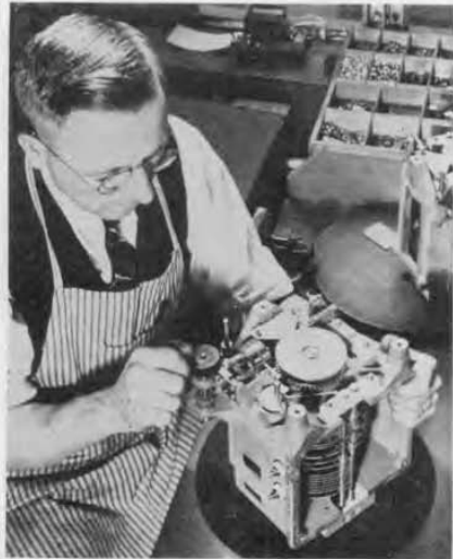
Figure 4. Final adjustments on a Type 622 "bath-tub" capacitor, a special model designed for mechanical stability under extreme conditions.
